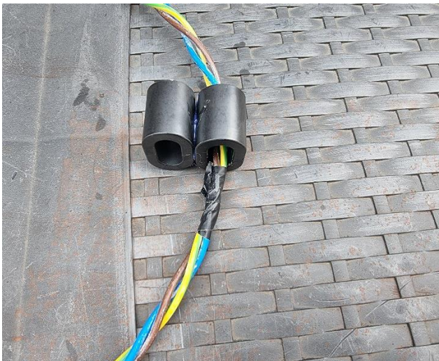
(STEP 1 leave 10 inch of cable below toroid)
