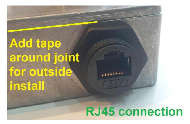
The relay unit has a RJ45 socket for the standard Cat cable connection, please ensure this is taped  $\!\!\!/$  sealed for external use.
