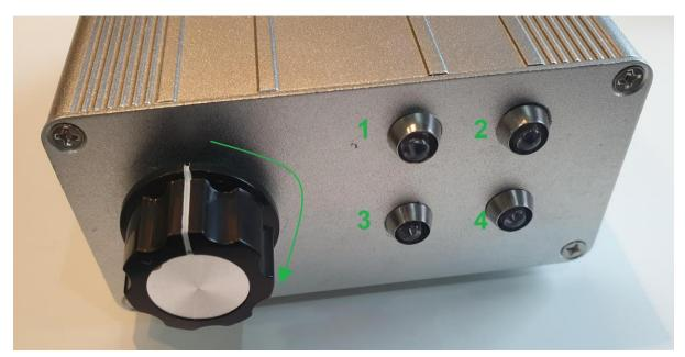
You rotate the switch clockwise to select from antenna port 1, 2, 3 and 4. You can see the port numbers on the image above.
