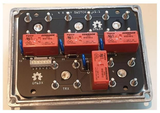
The PCB is attached to the lid. Short cables go from the RJ45 to the lid so please be careful if separating for drill mounting hole etc.
