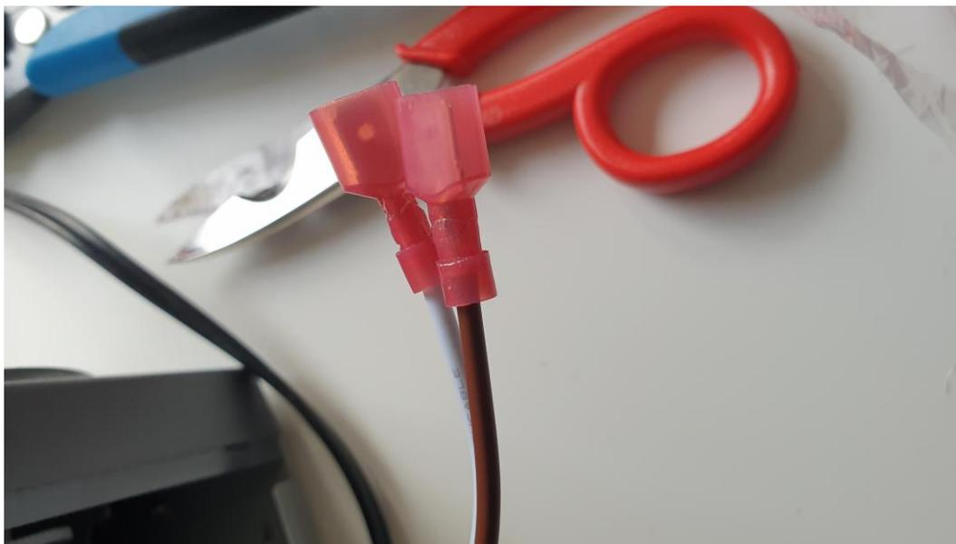
Now install the 2 x red crimp on spade connectors to the brown and white wire.
