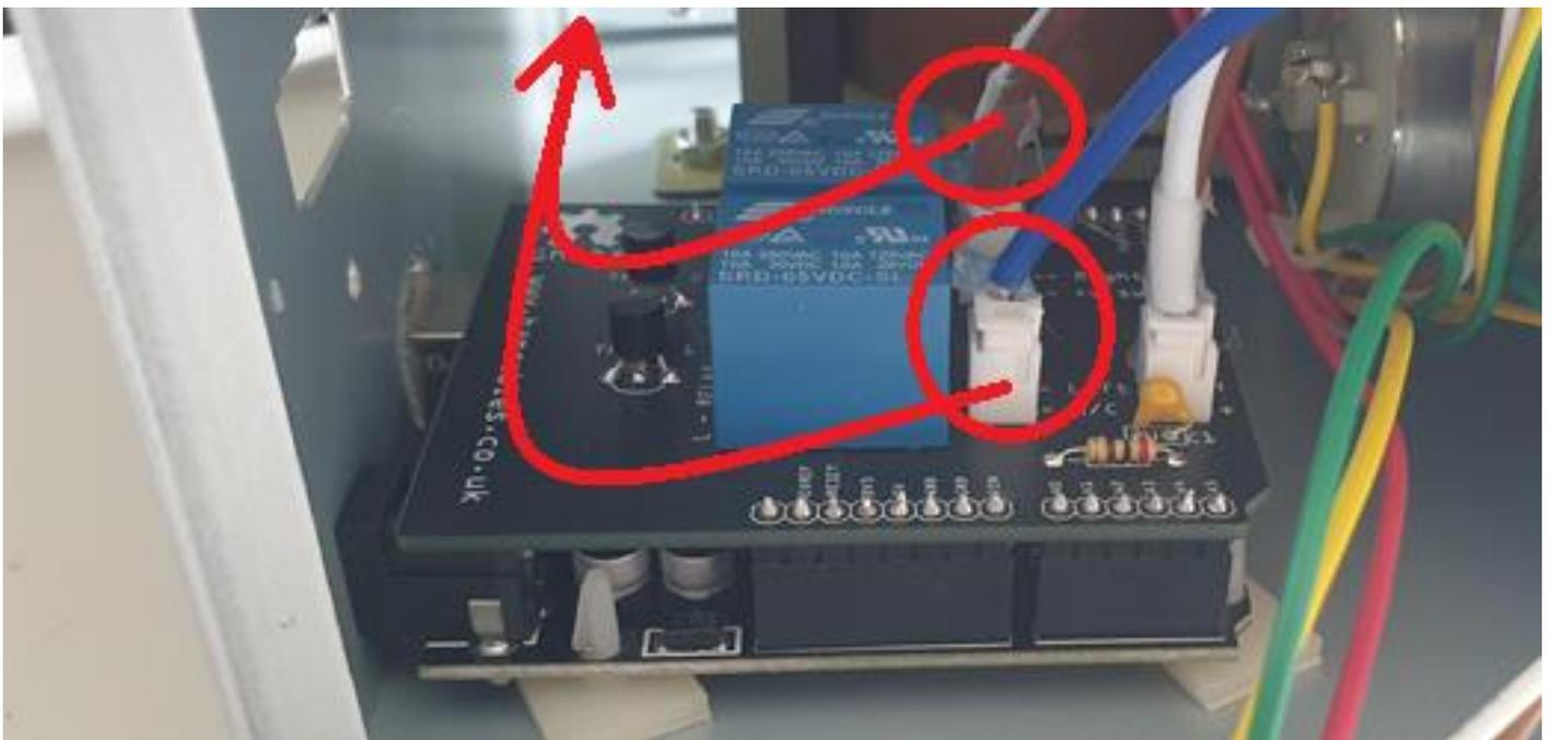
Now feed the white, brown and blue wires as shown through the space at the back over to the other side of the controller.
