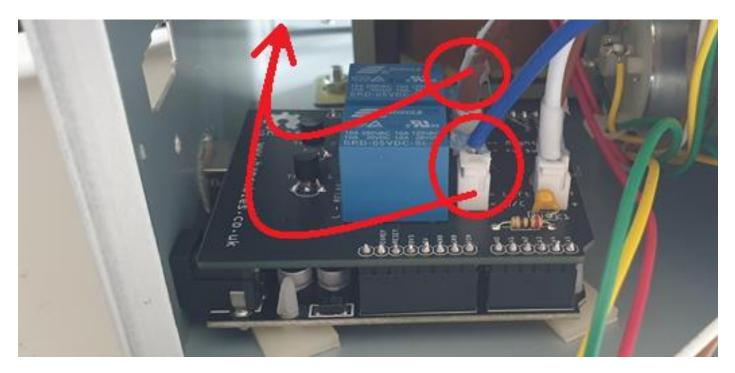
Now feed the white, brown and blue wires as shown through the space at the back over to the other side of the controller.
