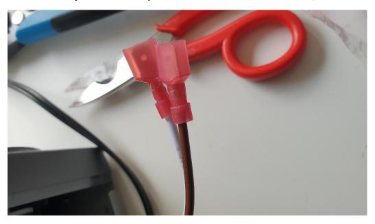
Now install crimp on spade connectors to the brown and white wire. (Or solder)
