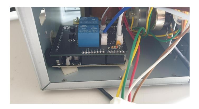
Now stick the USB controller down on the pads. I had to pull through the white 6 pin rotator cable connector, just to give some extra space to get my hand in when sticking it down. This is very easy as the connector has push in sides which allow it to be pushed back into the controller very easily.
