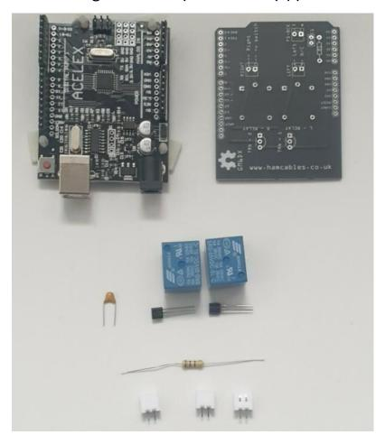
First step is to solder all the pieces on as per the photo. (2x transistors, 2x relays, 1 x resistor, 1x capacitor and 3x JST connectors).
