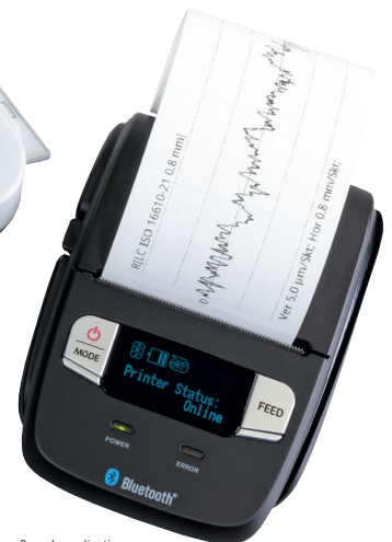
Sample application: MarSurf M 310 set with printer (order no. 6910267)
