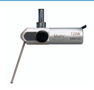
The inductive **T20W** probe is a universal device. The fact that the probe arm can be moved in a range of 180° and that there are a variety of clamping options for the probe means that measurements can also be performed in areas that are difficult to access. You can combine easily exchangeable probe arms with a variety of styluses in order to adapt the probe to the relevant measurement tasks or workpieces.
