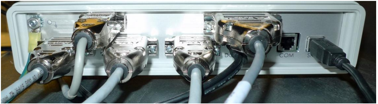
Figure 3. Rear of CSI box with cables connected. USB service cable (far right) is connected in this photo but is only required if using command interface described in section 5 of this manual.
