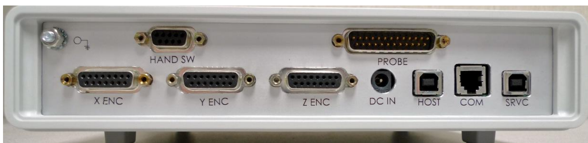
Figure 2. Rear of the CSI box (this photo is the Tesa/B&S version of CSI, TTL version will look different). Connect CMM cables to designated connectors prior to powering on the CSI box.
