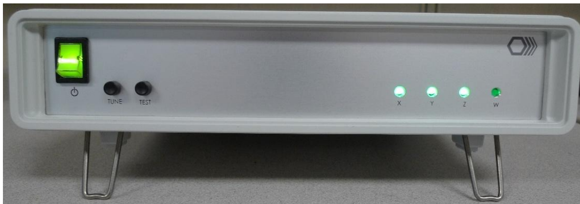
Figure 5. CSI powered on. The X,Y, and Z LED colors are dependent on the last “Auto Tune” operation that was performed.
