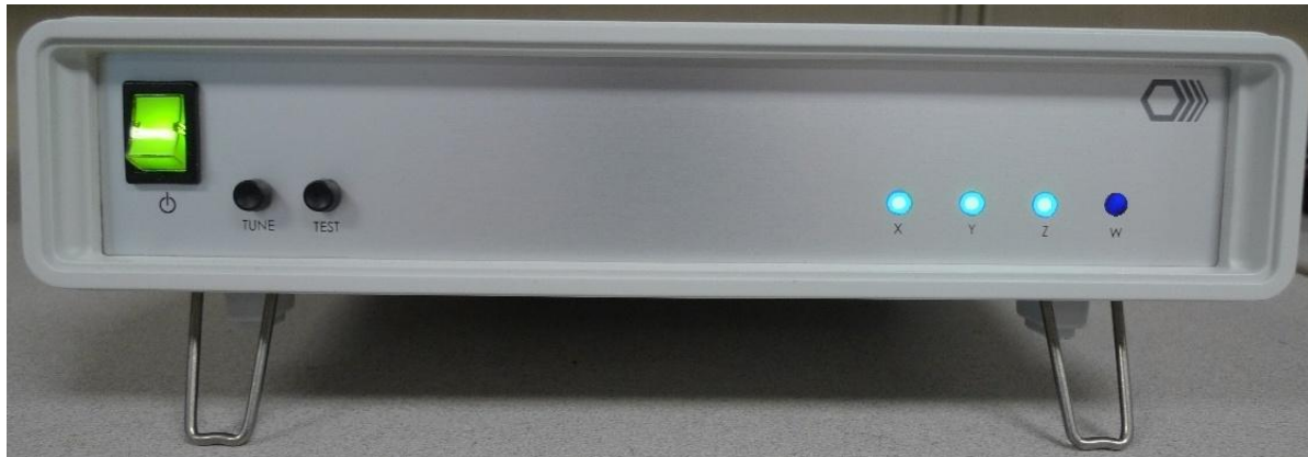
Figure 7. CSI box with all 3 LED's blue. The tune mode is set for “Tune all”.
