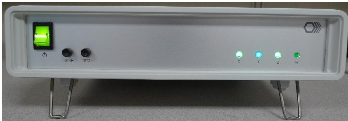
Figure 8. CSI box with “Y” axis LED blue. Tune mode is set for “Tune Y”.
