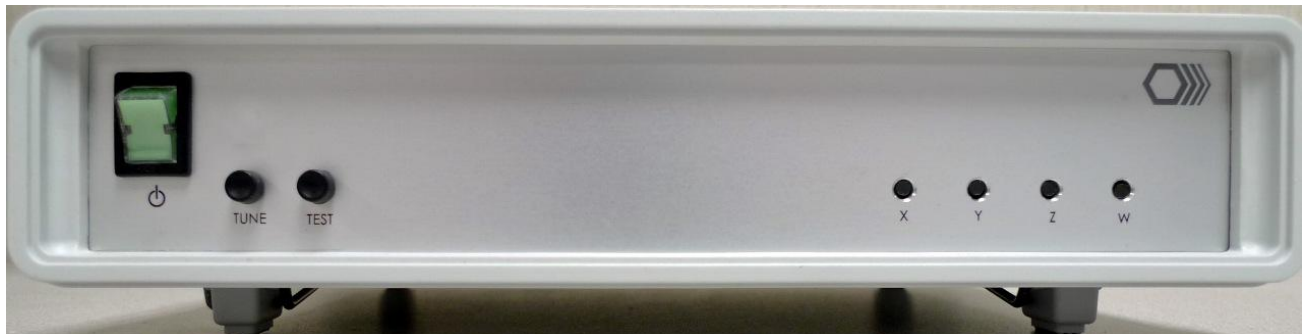
Figure 4. Front of the CSI box. Power switch is located on the far left. Photo is with the power switch in the “Off” position.
