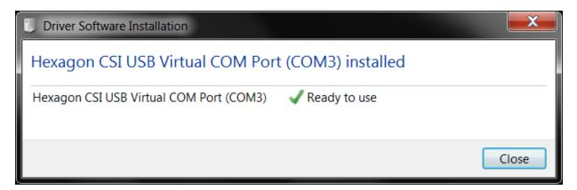
You can also check for the COM port number in device manager as shown here (COM 5 in this example)
