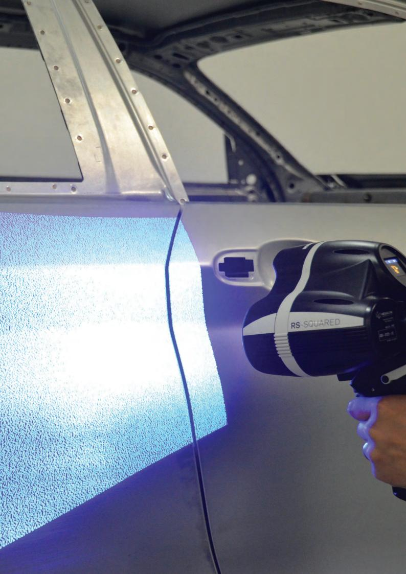
Often, the time needed to scan a part is the most important factor when planning measurement tasks. The part might only be available for measurement for a limited time or restricted to an inconvenient location. That's why Hexagon has created the RS-SQUARED Area Scanner, the world's first structured light scanner mounted on a portable measuring arm.
