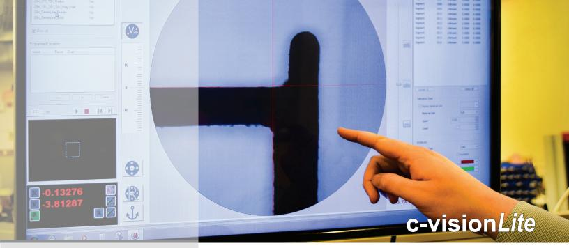
**c-vision** *Lite* is a manual, easy to use video comparator. Precision optics and vCAD electronic overlay charts make comparative inspections easy.
