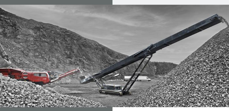
The Finlay® TC-80 mobile stockpiler is a highly mobile and flexible machine that offers operators an efficient, reliable and cost-effective stockpiling solution. The robust machine has been engineered for flexibility across a range of applications and features variable belt speed, adjustable feed height and variable discharge height.
