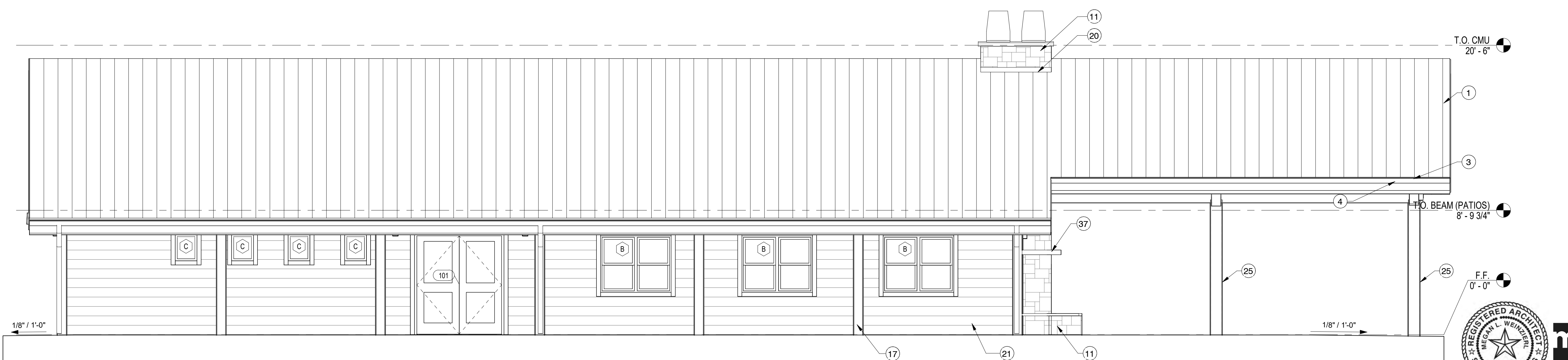
4 GATHERING LODGE BUILDING ELEVATION - SOUTH SCALE: 1/4" = 1'-0"
