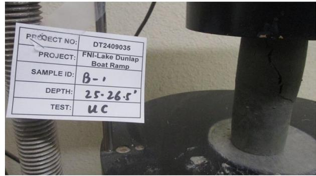
Failure Mode: Single Inclined Failure Plane
