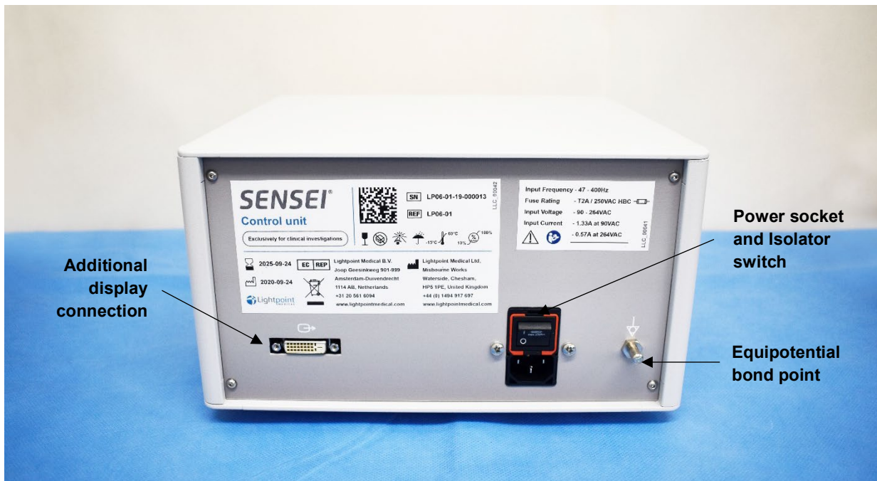
Figure 4 - Control Unit rear panel
