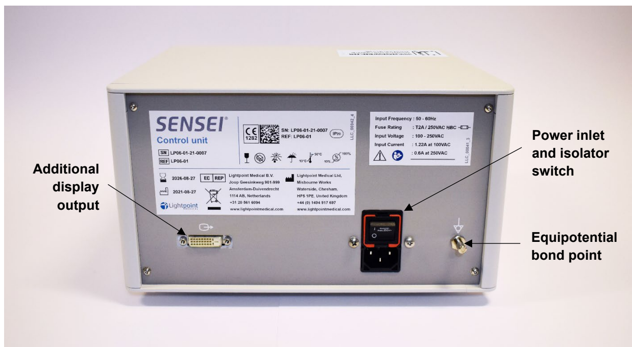
Figure 4 - Control Unit back panel
