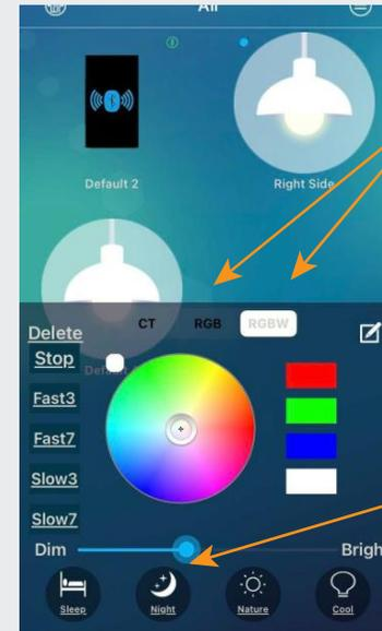
Dim Bar Used to increase or decrease the brightness setting of the grouping of fixtures, from 5% to 100% by sliding the bar.
