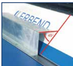
45° geometry on both sides of the upper beam gives you the advantage of being able to fold complex parts.
