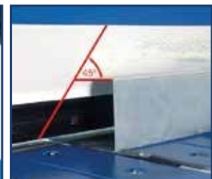
45° geometry on both sides of the upper beam gives you the advantage of being able to fold complex parts.
