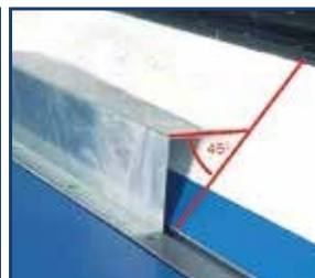
45° geometry on both sides of the upper beam gives you the advantage of being able to fold complex parts.
