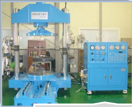
Hydraulic Test M/C
