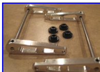
Sway bar set-Contains 4 arms, 2 steel torsion bars and 4 Delrin bush- ings. $50.00
