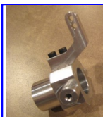
Steering knuckle (Includes 2 alumi- num knuckles, and 2 arms, and 4 bearings) $65.00 a pair
