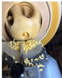
Excavating leaving a star point
