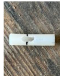
'Special' tube, 8mm OD, 6mm ID
