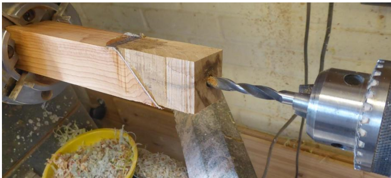
Drilling blank on lathe
