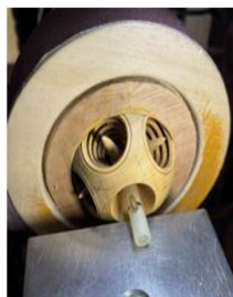
Measuring the star point length
