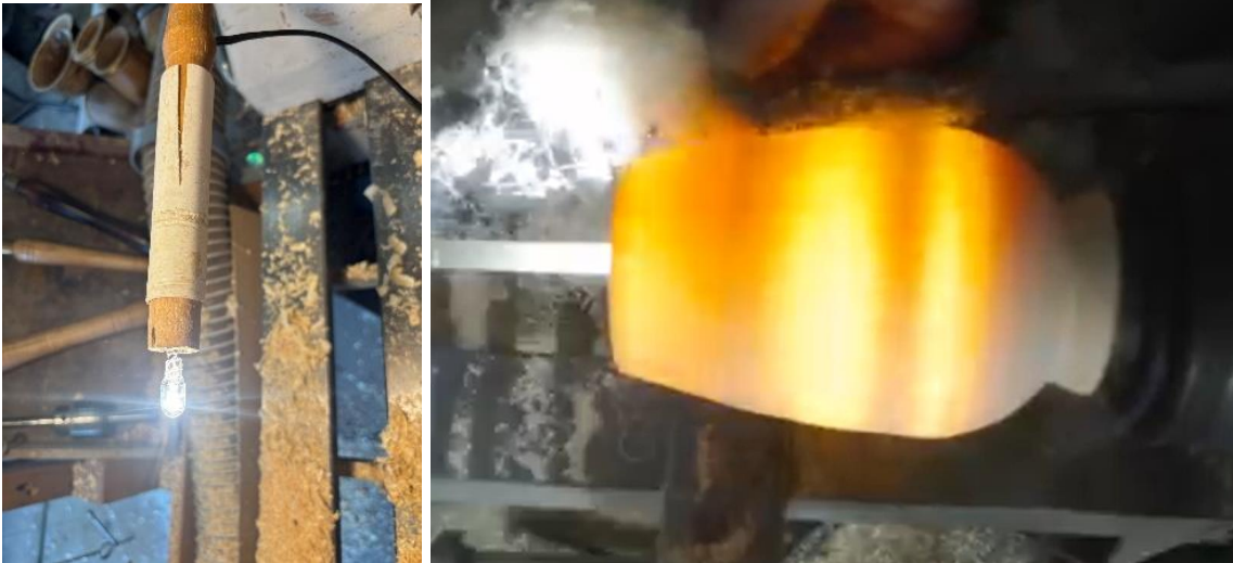
Picture: LED inspection light mounted to the tailstock, with a sliding cover. Action shot cribbed from Oliver's woodturning video, as I didn't take one!)
