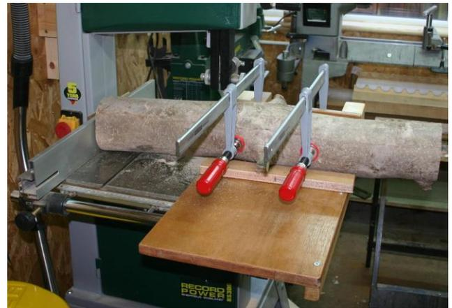
*Figure 38 (left) Jig used for small cylindrical and for (Figure 39, right) large cylindrical stock. The guide rail runs against the edge of the table ensuring a straight cut*
