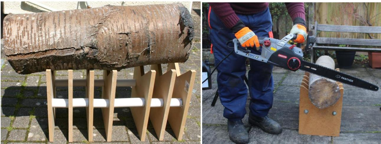
Figure 30 (Left) The chainsaw horse as built supporting a trunk of Cherry ready for cutting. Figure 31 (Right). Slicing a bole of Ash supported in the chainsaw horse.
