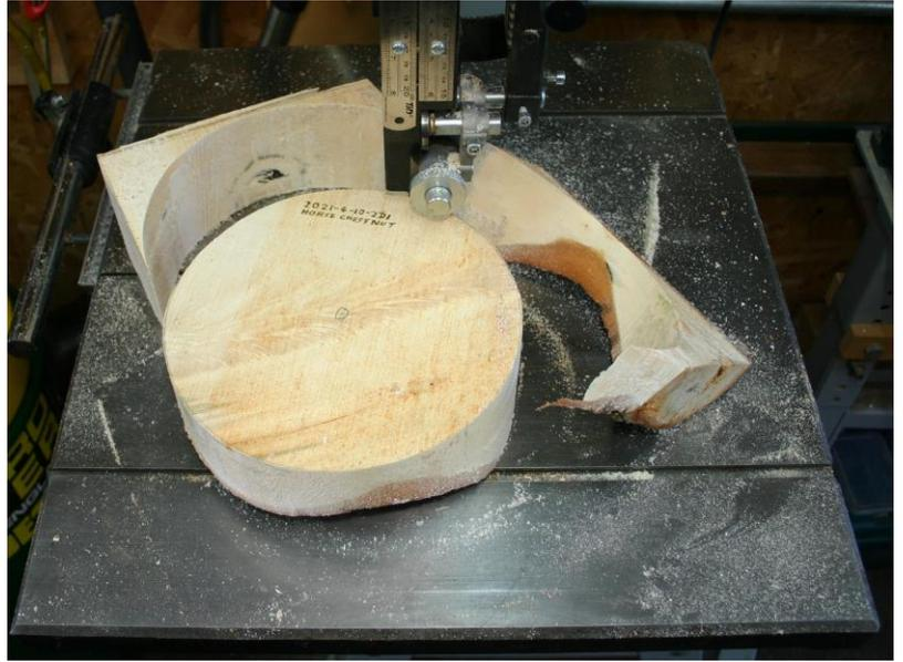
*Figure 33 (left). This Record Power BS300 model is a good size for a small workshop; 190 mm (7.5") depth of cut, 300 mm (12") throat width, mounted on castors for ease of movement. Figure 34 (right). A typical woodturner's use for a bandsaw, cutting out a bowl blank from some Horse Chestnut.*
