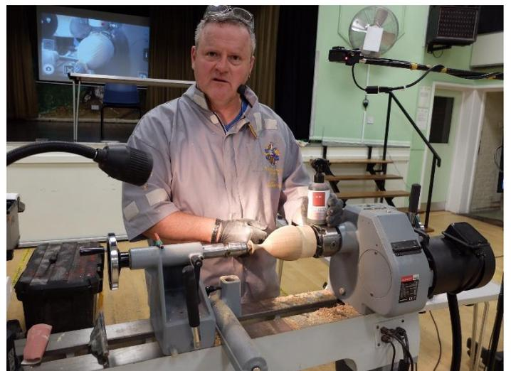
A round skew was used to cut the recess to fit the base disc as closely as possible. Once the walls were the desired thickness the corner of a skew was used to define the centre at the top of the hollowed space. This was important to ensure that a drill used to bore the neck would centre precisely.
