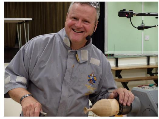
This was followed by sanding with 180 grit. Colour stain was applied with a brush. The spread of stain is best controlled by burn lines. The final stage of decoration was the application of liming wax followed by burnishing off the excess. The work was completed by turning a short finial of light wood to fit in the top and by gluing in the bottom.
