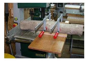
Figure 38 (left) Jig used for small cylindrical and for (Figure 39, right) large cylindrical stock. The guide rail runs against the edge of the table ensuring a straight cut
