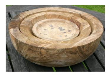
Figure 24 (left). The large rough sawn end-grain blank mounted on the lathe (by means of a faceplate) ready for turning. Figure 25 (right). Three rough turned bowls were produced by coring out with a Bowlsaver.
