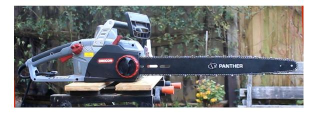
Figure 28. Here the Oregon saw has been fitted with a longer 50cm (20") guide-bar running thinner gauge 0.043" Panther mini chain. It's essential to **GET EXPERT ADVICE** if changing from default bar/chain to ensure it is safe to do so. The reason for changing was to improve performance when the saw is fitted to a portable chainsaw mill (Figure 45) otherwise the default shorter bar and chain was totally adequate in performance.
