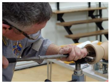
cleanly using a spindle gouge presented horizontally with the bevel parallel to the direction of cut. A spigot 3/8 - inch wide was then cut, to define a disc which would become the bottom of the hollow form. Some decorative rings were cut and the surface sanded and finished. Next this disc was parted off with a narrow parting tool leaving a small witness ring to define the wall thickness.
