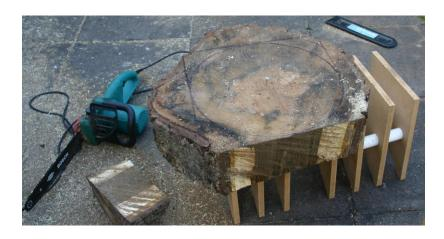
Figure 23 (left). The 12" ruler demonstrates the large cross-sectional diameter of the slice across the Walnut trunk. Figure 24 (right). An exploratory cut on the side of the trunk revealed sound (brown) heartwood and cream-coloured sapwood.
