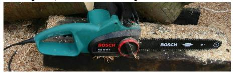
Figure 26. Bosch AKE 40-19 S, 1.9Kw corded electric chainsaw with a 40cm (16") guide-bar running 0.043" gauge chain (that's thin to maximise performance).
