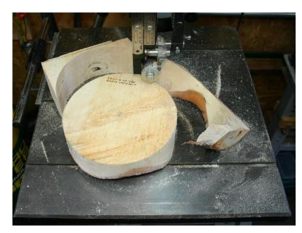
Figure 33 (left). This Record Power BS300 model is a good size for a small workshop; 190 mm (7.5") depth of cut, 300 mm (12") throat width, mounted on castors for ease of movement. Figure 34 (right). A typical woodturner's use for a bandsaw, cutting out a bowl blank from some Horse Chestnut.
