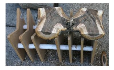
Figure 31 (top left). Here the horse is supporting a Walnut crotch (also shown in Fig. 22), for longitudinal slicing.
