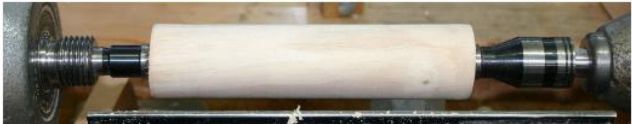
5. After removing the bark and irregularities with the spindle roughing gouge, the Holly showed no cracks or other defects.
