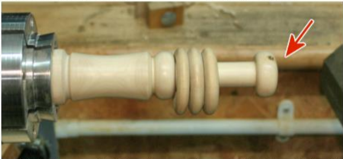
15. With the rings completed, the rattle can now be mounted in a 35mm chuck, using a spigot cut in waste wood at the left of the rattle, to enable final shaping and removal of waste wood using a spindle gouge at the right hand end (arrowed).
