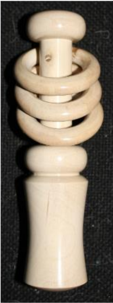
17. The completed Holly rattle after final sanding, sealing and buffing.
