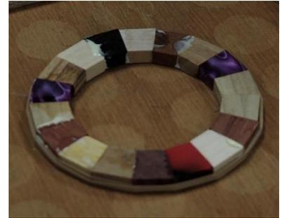
The angles must be cut very precisely – the smallest error is multiplied by the number of segments to result in an unacceptable misfit when gluing up. The best approach is to make a cutting sledge (see image on left) which slides on the table saw (Ben is willing to supply details or various designs are available on-line). The saw blade must be sharp and ideally of thin kerf. Initially, trial runs must be made, adjusting the angle until the pieces form a perfect circle.
