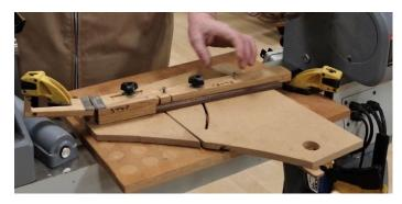
unacceptable misfit when gluing up. The best approach is to make a cutting sledge (see image on left) which slides on the table saw (Ben is willing to supply details or various designs are available on-line). The saw blade must be sharp and ideally of thin kerf. Initially, trial runs must be made, adjusting the angle until the pieces form a perfect circle.
