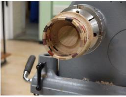
clamped and left overnight. The bangle was then turned to its final size using a gouge on the outside and a scraper on the inside. The edge was rounded with sandpaper.
