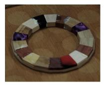
The angles must be cut very precisely – the smallest error is multiplied by the number of segments to result in an
