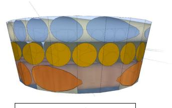
2D Sketchup Model of the dowel patterns and shape determined by the dowel layers and cut.
