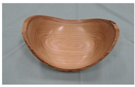
have a 300mm straight tool rest, which is a bit hard to get in a convenient position. I sanded the inside using drill/arbor and finished the same as the outside. Although there are noticeable marks still visible and the decoration in the recess are largely sanded away, I'm happy that it represents where I am in my learning journey.
