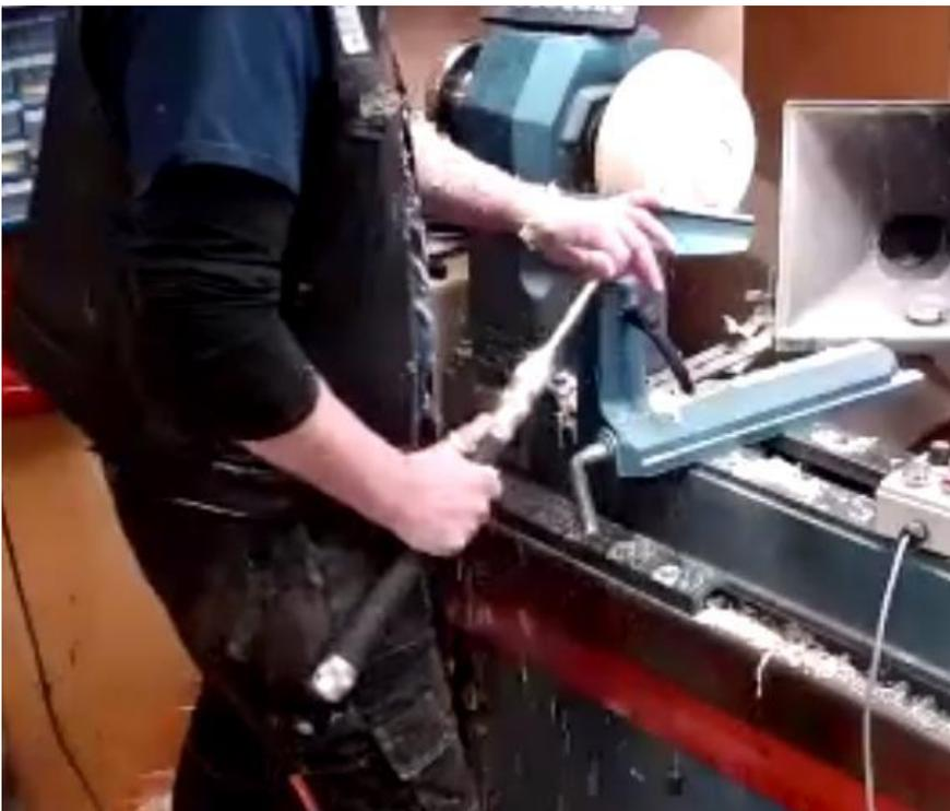
There was some discussion about the relative merits of push and pull cuts, but the significance of grain direction was not made clear. It was shown that a cleaner cut is obtained by keeping the gouge handle low, so making a slicing action see image to left.
