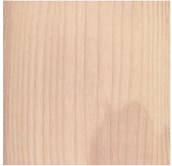
Heartwood is rated as perishable, or only slightly durable in regard to decay. Ash is also not resistant to insect attack. Generally easy to turn and finish – very commonly used at fairs by demonstrators.
