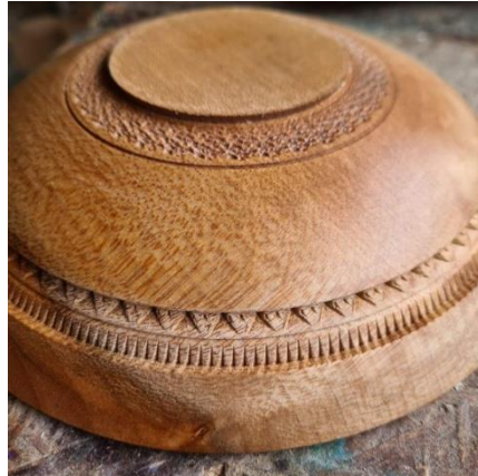
Texturing done using Sorby Rotary Texturing and Spiralling Tool
