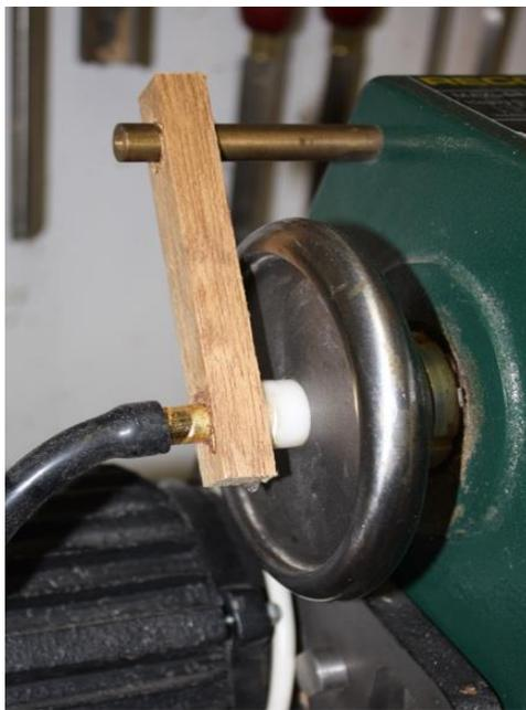
So, for a bowl 10 inches diameter the area is 78.5 sq in. and with just 2 pounds per sq in. there will be some 150 pounds force to hold the work in place. Since a vacuum cleaner shifts a large volume of air, the system does not need to be very leak-proof.
