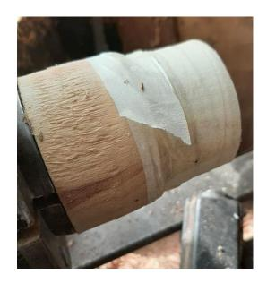
A **jam chuck** mounts in the **lathe** headstock and provides a friction-fit cavity or surface that the turning can "**jam**" against. Each jam chuck may well be turned specifically turned to a
