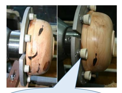
Stacking Studs have been added in this version to give extra height to the rubber buttons. These can also be used on their own without the rubber buttons.
