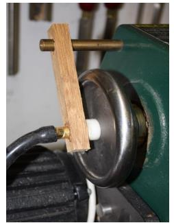
So, for a bowl 10 inches diameter the area is 78.5 sq in. and with just 2 pounds per sq in. there will be some 150 pounds force to hold the work in place. Since a vacuum cleaner shifts a large volume of air, the system does not need to be very leak-proof.
