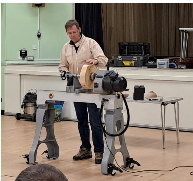
A suitable sized tenon is turned first. Normally we would recommend a diameter just a little larger than the diameter of the chuck for best grip but in this case we need to be larger again as we expect that after drying, the distortion of the bowl will be reflected in the tenon as well and so the tenon will also need truing up to a circle before it can be remounted, The centre of the tenon is marked for later
