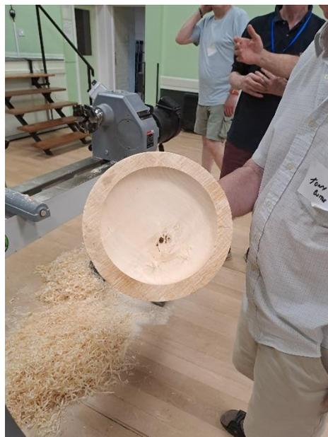
Once the moisture level has dropped sufficiently the bowl can be remounted – probably with a Longworth chuck or similar and the tailstock brought up on the centre mark you left earlier. The bowl can then be finished in the normal way
