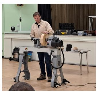
A suitable sized tenon is turned first. Normally we would recommend a diameter just a little larger that the diameter of the chuck for best grip but in this case we need to be larger again as we expect that after drying, the distortion of the bowl will be reflected in the tenon as well and so the tenon will also need truing up to a circle before it can be remounted, The centre of the tenon is marked for later
