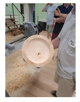
Once the moisture level has dropped sufficiently the bowl can be remounted – probably with a Longworth chuck or similar and the
