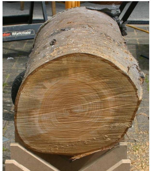
*Figure 6. Above Trunk of Cherry with extremity shrinkage cracks. RIGHT The same trunk after cutting back a few inches revealing sound wood.*
