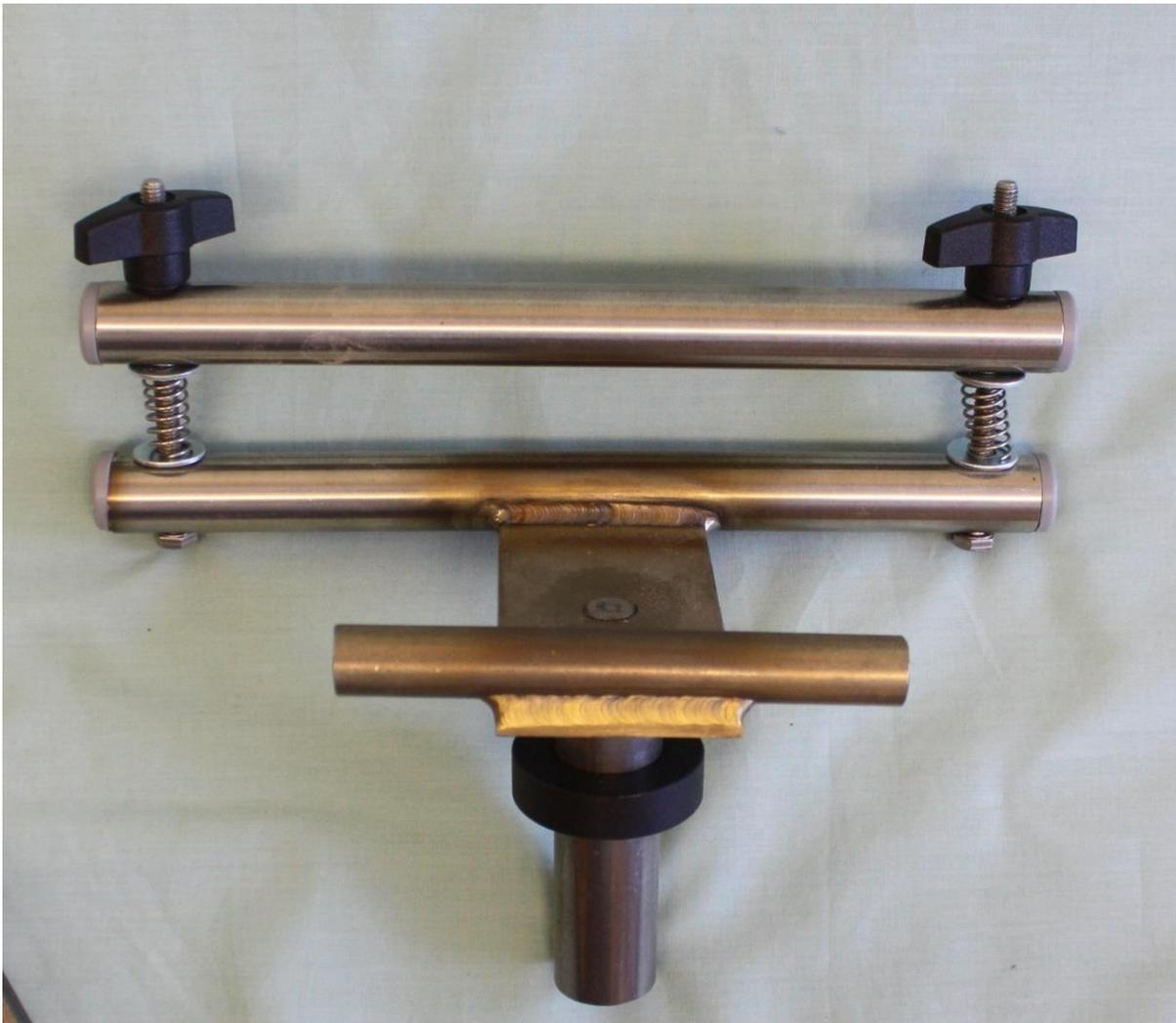
Robert Sorby have also recently introduced a hollowing jig of similar principle, but this has only a single restraining bar. It does not include the hollowing tool itself and has no provision for a laser thickness guide.
