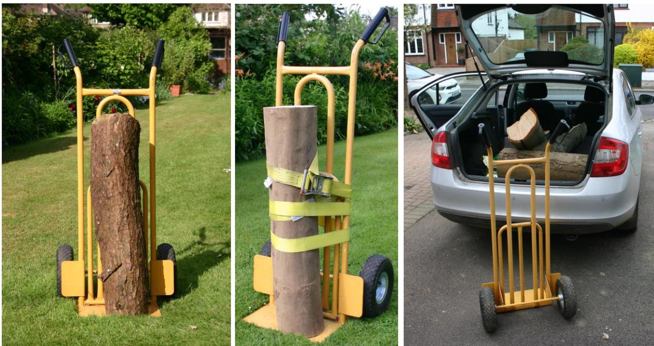
*Figure 5. Using a sack truck for handling heavy boles and boughs. A section of trunk can be tipped on end and then fairly easily tilted to allow insertion of the sack truck platform underneath. If necessary the trunk can be further secured as shown using a ratchet strap. It is then an easy task to wheel and transfer the wood to the car for transport back to base.*
