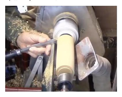
After remounting one end, a lid was parted off from one end leaving about 110mm for the body. A beading tool is used to put a 3mm bead at the bottom.
