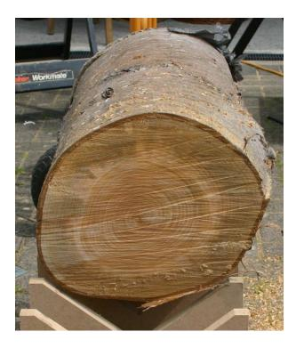
Figure 6. Above Trunk of Cherry with extremity shrinkage cracks. RIGHT The same trunk after cutting back a few inches revealing sound wood.
