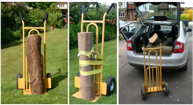
Figure 5. Using a sack truck for handling heavy boles and boughs. A section of trunk can be tipped on end and then fairly easily tilted to allow insertion of the sack truck platform underneath. If necessary the trunk can be further secured as shown using a ratchet strap. It is then an easy task to wheel and transfer the wood to the car for transport back to base.
