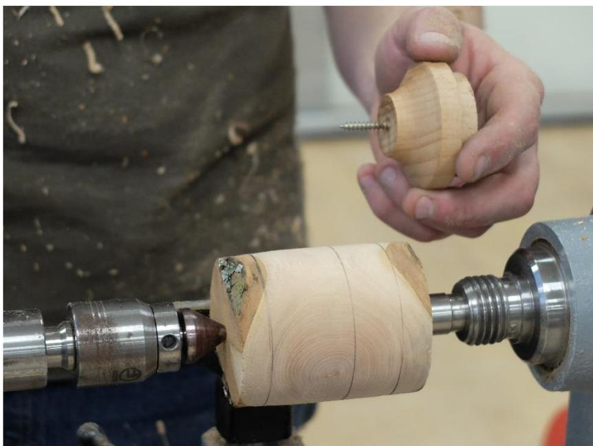
Before the final shaping the blank is removed a special screwchuck is used to mount it as can be seen in the photo.
