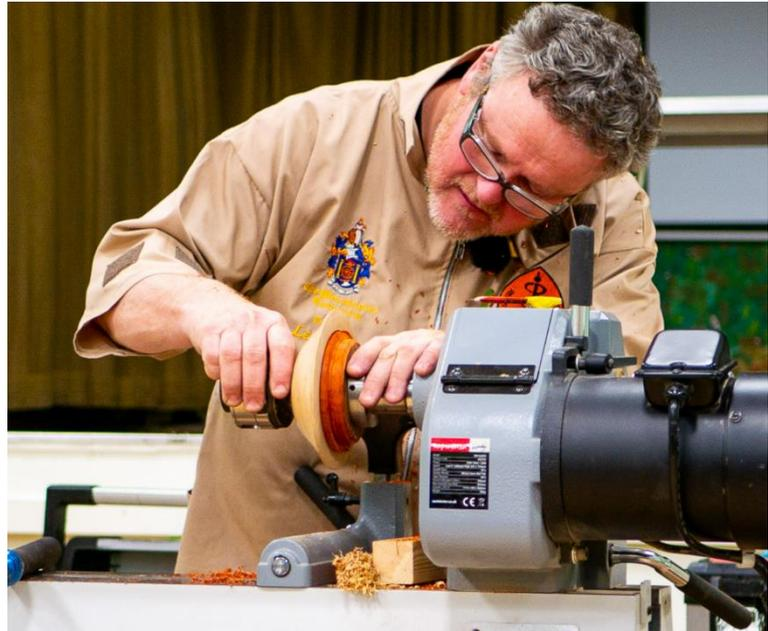
The final stage was to complete the hollowing, finishing with a small sharp gouge. Les prefers wet sanding using lemon oil as lubricant.
