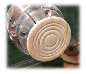
I cut a piece of wood, from the original stock, adjacent to the piece I used for the vase in the hope the grain of the insert would match. I debated with myself whether to colour the insert, or carve it or indeed use a different wood. Eventually I settled on plain wood and added the rings for decoration and to (maybe) confuse the eye regarding the grain.
