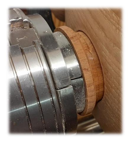
I made a jam chuck to fit the register in the front of the vase and reversed the vase to remove the chuck foot.
