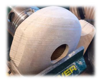
I've bored through the side and started hollowing out. At this stage I thought it might be good idea to give some form to the outside; mainly to feel how thin I was going! I removed the wood with a micro-plane and then sanded.
