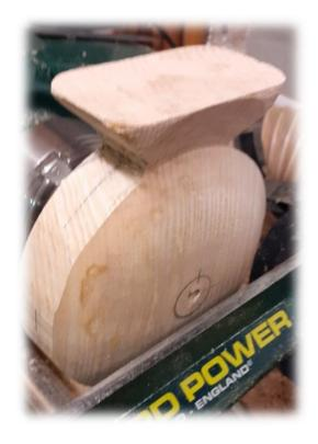
With the work reversed and held in the chuck the profile on the front is turned to match that on the reverse.
