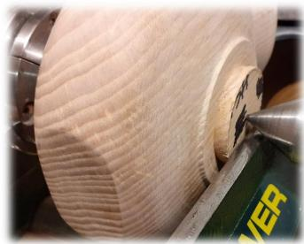
Foot was removed and face blended with initial turned surface. Face then finish sanded. I removed the foot remnant off the lathe with a carving tool. Plus a bit of sanding.
