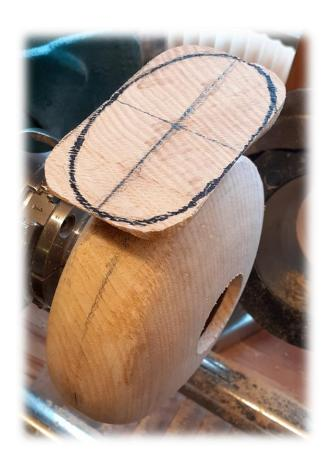
I also roughly marked out the shape of the neck lip, but made the mistake of using a "Sharpie", which penetrated the wood a little too much. I would just use pencil next time!
