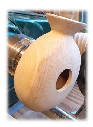
I had trouble determining the thickness of the face nearest the chuck. I didn't want to go through and I didn't want it too thick (though it probably doesn't matter). To give me some indication, I measured the overall thickness as best I could (as the chuck was in the way), then subtracted the measurement from the front face to the back of the hole.
