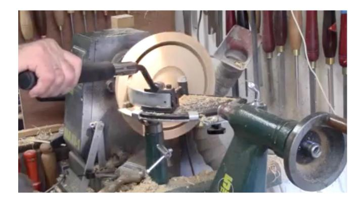
The outer bowl is removed from the chuck and the centre part remounted on the chuck in expansion mode. This permits a foot and chucking point to be cut (for a smaller chuck).
