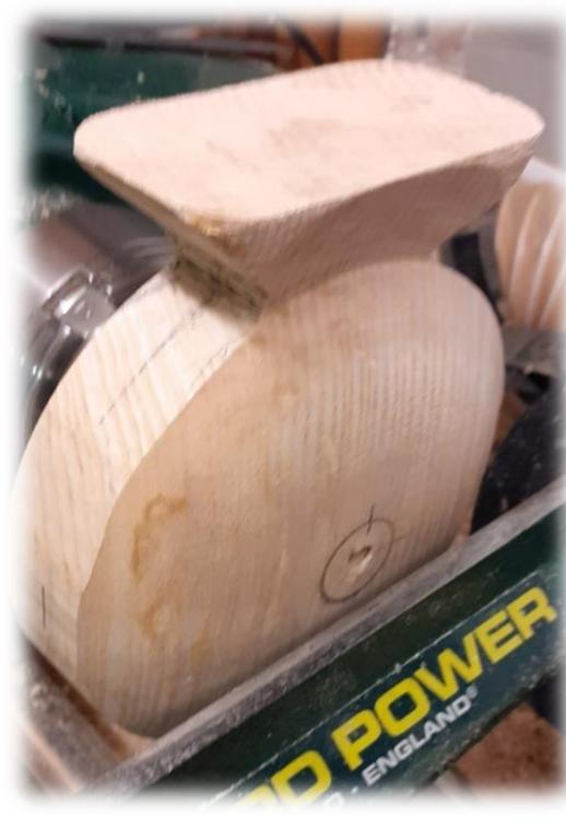
With the work reversed and held in the chuck the profile on the front is turned to match that on the reverse.
