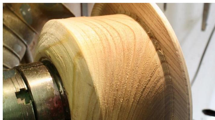
Using a light behind to show the thickness clearly, the rim is thinned to 3mm. The hat is also hollowed at this stage.
