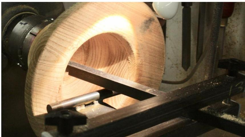
Using my hollowing jig, the hollowing is completed.
