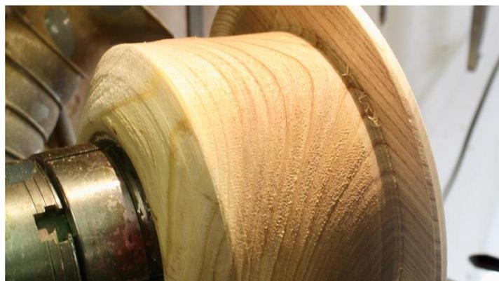
Using a light behind to show the thickness clearly, the rim is thinned to 3mm. The hat is also hollowed at this stage.
