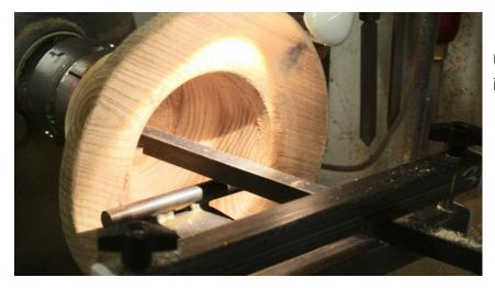
Using my hollowing jig, the hollowing is completed.
