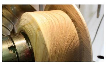
Using a light behind to show the thickness clearly, the rim is thinned to 3mm. The hat is also hollowed at this stage.
