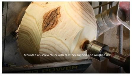
The block was then mounted by the tenon at the crown end using dovetail jaws and the bottom flattened. This end will be the rim of the hat. The rim is then developed and the crown reduced somewhat.
