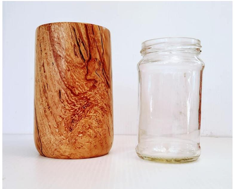
This particular piece of very punky spalted beech (from Jason's Wood Craft) was a nightmare turn. The thinner I went the more it warped due to the stress relief between the punky & the harder wood. This made it really difficult to finish despite a couple of hours shear scraping & sanding (to 600 grit), especially the inside which I admit I gave up on.
