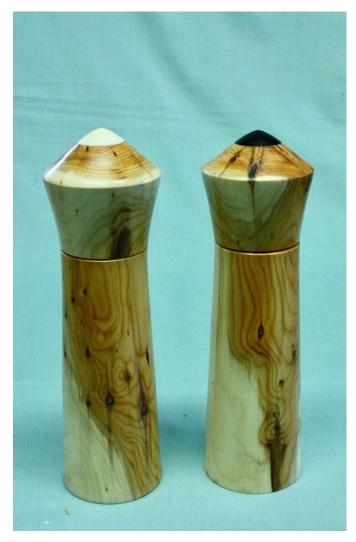
The choice of mechanism comes first. The cheaper versions cost about £5 each and have the adjusting screw nut at the top. The so-called crush/grind mechanism is rather expensive at about £12 each, but I strongly recommend it because it last for years and allows for a wide range of designs. If you are
