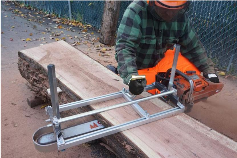
*Figure 39. A portable chainsaw “Alaskan” Mill in use with a petrol driven chainsaw slicing a large trunk of wood.*
