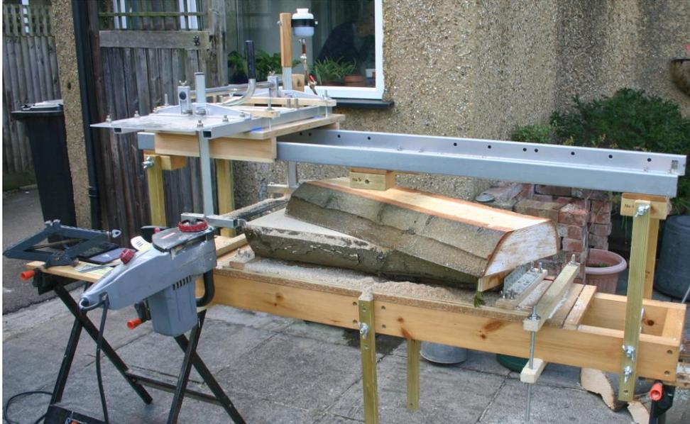
*Figure 45. The portable chainsaw mill fitted with the 20" guide bar in use with Horse Chestnut being milled on the home built jig*
