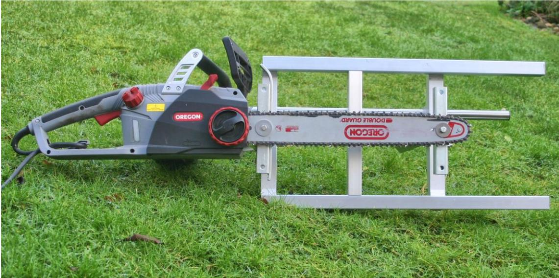
*Figure 43. Here the CS1500 chainsaw is attached to the portable chainsaw mill by means of two (M6 & M7) bolts through the guide bar into the clamps of the mill. This is shown with the default 45cm guide bar as supplied with the saw*
