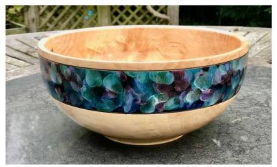
The outside of the bowl was sealed and sanded to 320 grit. Pencil lines were drawn to define the strip to be painted and masking tape applied carefully to these lines. Two coats of ebonising lacquer were applied. Once fully dry, Jo Sonja paints were applied in random dabs, which were then blown around with a compressed air jet.
