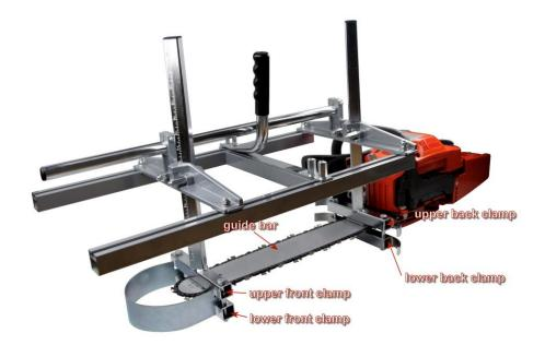
Figure 41. A conventional petrol driven chainsaw is easily attached to the mill frame (as shown here) by means of two sets of clamps which grip the chainsaw guide bar. The problem with an electric chainsaw is that the guide bar is too slim and the clamps overlap the running chain.
