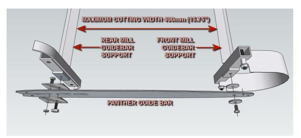
Figure 42. CAD drawing showing how the clamping problem was solved by dispensing with the clamps and bolting the guide bar to the mill instead. The 20" Panther guide bar mounted in the mill gives a maximum cutting width of 400mm
