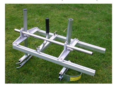
Figure 40. The Royston 24 inch capacity "Alaskan" Portable Chainsaw Mill.
