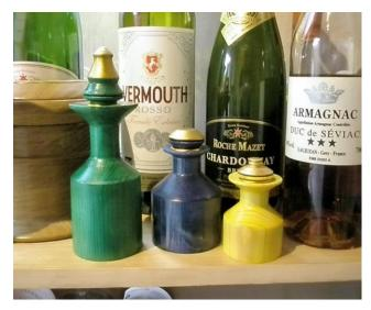
Turning the shapes was relatively easy but quite dusty due to the age of the timber. I drilled a hole in the top end with a 22mm forstner bit to take the candle cups that were superglued in place, then spirit stains were used on the wood before sealing the bottle shapes with acrylic sanding sealer. Finally a light coat of acrylic gloss spray was applied before a light polish.
