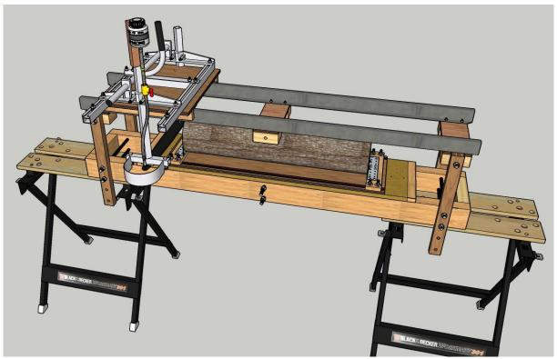
Figure 44. CAD drawing of the jig designed to support the saw, mill and wood in use. The chainsaw plus mill is mounted on a carriage which uses furniture castors to run along two steel rails. An important feature is an auxiliary oiler to deliver chainsaw oil to the guide bar during operation. This is essential to ensure that the chain plus bar don't overheat in use.
