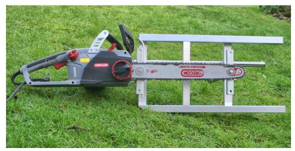
Figure 43. Here the CS1500 chainsaw is attached to the portable chainsaw mill by means of two (M6 & M7) bolts through the guide bar into the clamps of the mill. This is shown with the default 45cm guide bar as supplied with the saw
