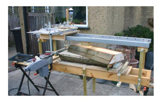
Figure 45. The portable chainsaw mill fitted with the 20" guide bar in use with Horse Chestnut being milled on the home built jig
