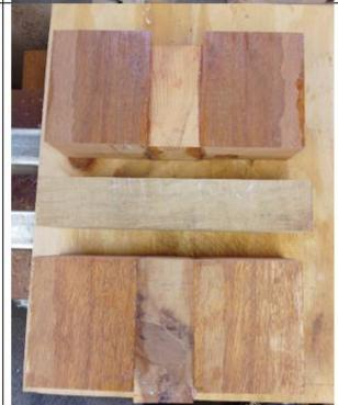
All the pieces glued together ready to cut into a circle for turning.
