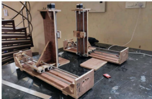
CNC machine(Computer Numerical control) designed to help build wings, fuselage, vertical stabilizers and horizontal stabilizers within days instead of weeks.
