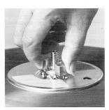
Threading of tape: Thread tape according to illustration below. The tape must be threaded neatly around the two tape tension arms (3) / (4). Thread leading tape end onto right-hand reel and manually rotate the take-up reel in a counter-clockwise direction until the tape is locked. Tape fitted with a transparent leader should be wound forward until the start of the magnetic surface has passed the heads. Set tape counter to zero by pressing the reset button (2).
